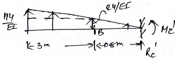
$$\begin{aligned} M_B' &= \frac{1}{EI} \times (24) \times 3 \times \frac{3}{2} + \frac{90}{EI} \times \frac{1}{2} \times 3 \times \frac{L^3}{3} \\ &= 378/EI = \Delta_B \end{aligned}$$
