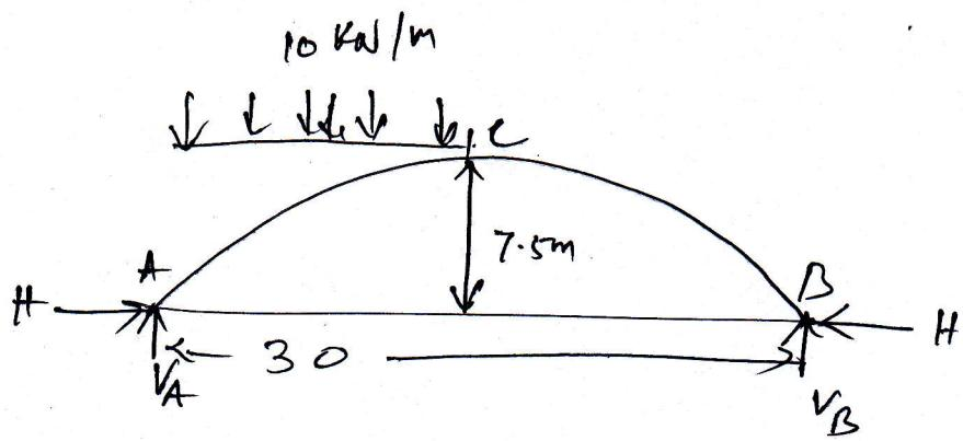
$$V_A = 112.5 \text{ kN}, \quad V_B = 37.5 \text{ kN}$$
