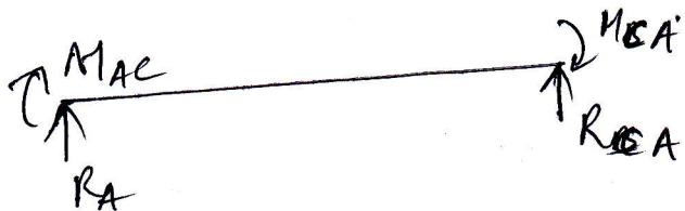
$$R_A = 3.6 \text{ kN}, \quad \text{similarly, } R_B = 3 \text{ kN}$$
