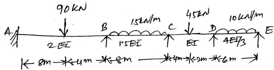
$$\text{FDM, } M_{AB}^F = -80 \text{ kNm}, \quad M_{BA}^F = +160 \text{ kNm}$$
